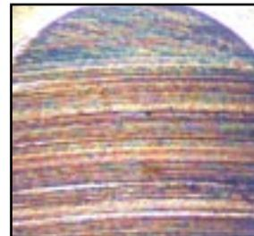
Other oils show adhesive wear and grooving caused by oil breakdown
